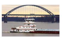
Helen Merrill, the last in a series of five pushboats, is powered by a pair of KTA50s. Electrical requirements are met by a pair of 99 kW MDDCR generator sets.
