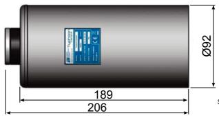
Shows standard aluminium alloy housing Not to scale, dimensions in mm.
