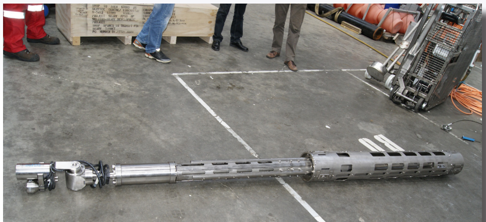
Camera, lights, pan & tilt, control system and fully extended deployment frame
