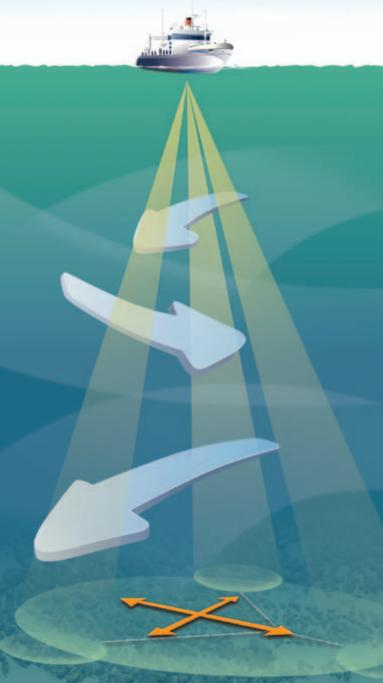
The FURUNO CI-88 is a new Doppler Sonar Current Indicator designed for every type of fishing vessels and hydrographic survey vessels. The high-definition 10.4" color LCD continuously presents tide speed and direction at three depth layers simultaneously in addition to ship's speed and drift. This variety of current information allows you to predict net shape and plan when to throw your net.
