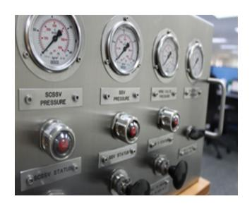
**The Well Control Panel** is a pneumatic/hydraulic control unit designed to safely operate the three main safety valves(WV, SSV & SCSSV installed on a producing well. Not limited to this, it is also used to operate other actuators and valves. The unit can be sized in accordance to customer's requirements to control the number of wellheads.
