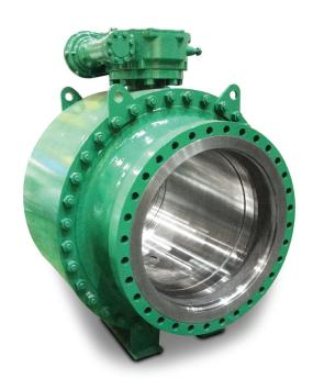
Split-body construction allows the use of forged materials in various grades of carbon steel, stainless steel, and high alloys, equipping the valves for some of the most severe service conditions.
