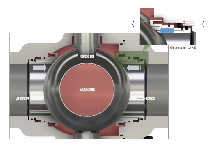
On request, the seat rings design may be modified to perform the "DOUBLE PISTON EFFECT" action.
