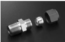
Dk-Lok Z Series single ferrule tube fitting is designed and manufactured to the highest quality standards. This fitting includes single ferrule with standard Dk-Lok fitting body and nut. To help identify Dk-Lok Z series from Dk-Lok Tube fitting, nut is black Molybdenum Disulfide (MoS2) coated.
