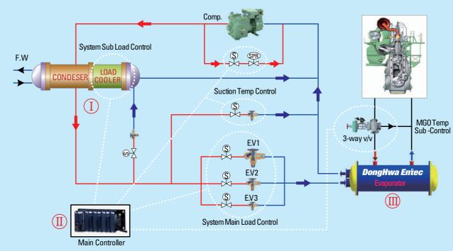
Remark: 3-Way valve will be applied to system as option depending on the required control accuracy of MGO outlet temperature.
