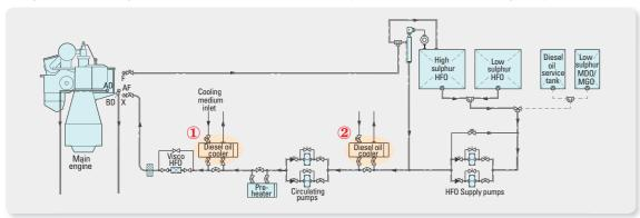
2. The cooler can also be installed before the circulating pumps. The advantage in this case is that the viscosity regulation may be optimized for both the engine and the circulating pumps.
